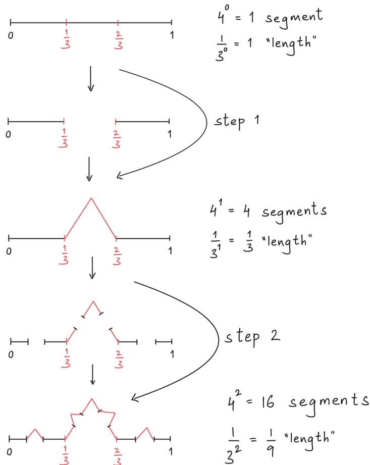
Figure 1: Procedure to construct the von Koch curve
